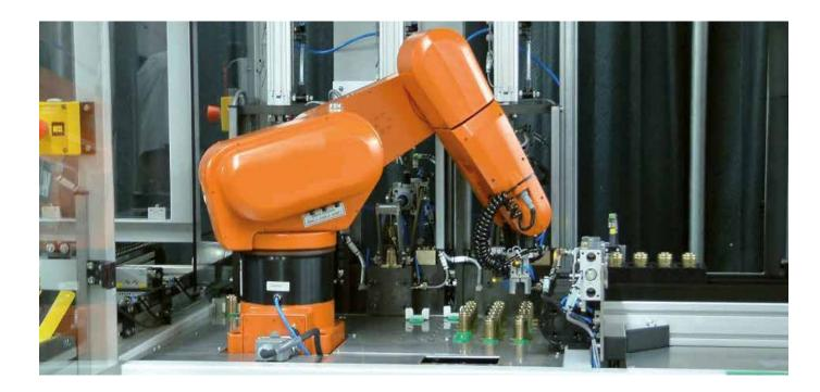
The system consists of two autonomous conveyor belts, each with one loading section, 20 pallets, 3 test stations with drainage device as well as an unloading section with trays. All test stations with clamping devices feature identical designs. The test consists of the following individual tests: Piston setting, operation test, leakage measurement and characteristic curve determination. At the end of the test, the valve tested is drained as far as possible.
