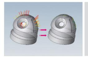
FormControl Best-Fit mathematically orients the workpiece in space in such a way that the measuring points match the CAD model as exactly as possible. Thanks to the individualised weighting of the measuring points, systematic measurement errors are compensated.
