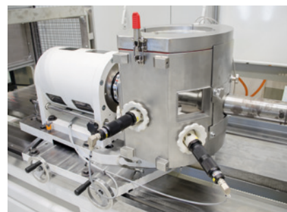
Test cavity with temperature sensors
