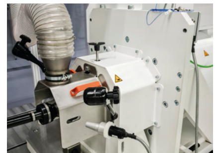
Swivel unit with temperature sensor
