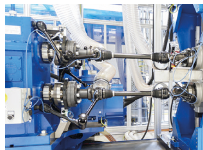
Air flow simulation and temperature measurement
