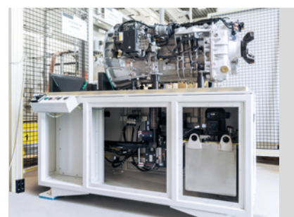
External oil drain station
